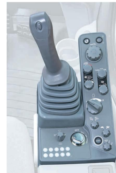
A dial type multi-functional controller makes operation easy and intuitive. Frequently used switches are located on the right hand side console panel within easy reach of the operator.
