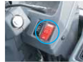
Electronically operated parking brake A simple press of a button sets and releases the parking brake.
