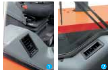
Front 1 and rear 2 defrosters reduce fogging for clear visibility
