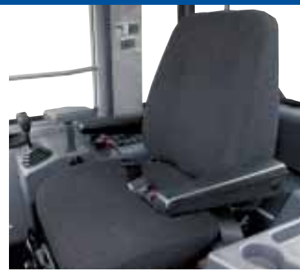
Deluxe suspension seat The comfortable cloth-covered seat offers both suspension and reclining adjustment.
