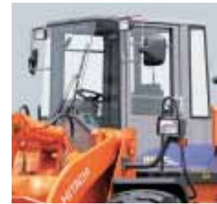
ROPS/FOPS* cab This rigid cab is ready "just in case" to help protect the operator from falling objects or during a rollover. The rear-hinged door makes entry and exit easy.
