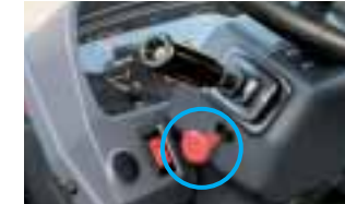
Shift lever lock Can be easily set to prevent accidental operation of the shift lever.
