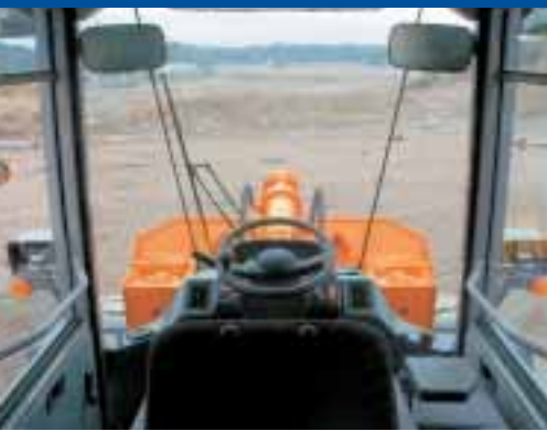
Clear view from cab front A pillar-less design gives an unobstructed view of the front.
