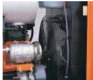
Fully enclosed engine fan guard A guard completely encloses the engine fan.
